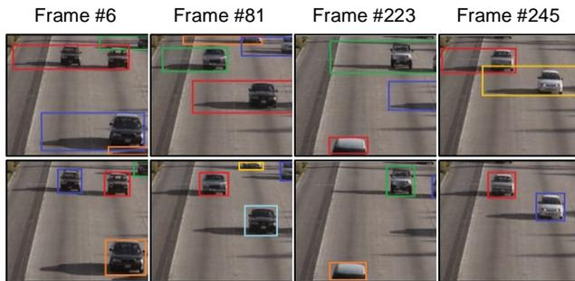
Fig. 4. The tracking results on "highway I" video sequence first row: without shadow removal, second row: with the proposed algorithm
