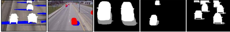
Fig. 3. The results of running the proposed system on different video sequences during daytime: original frame, shadow detection result, ground truth image from top to bottom, respectively
