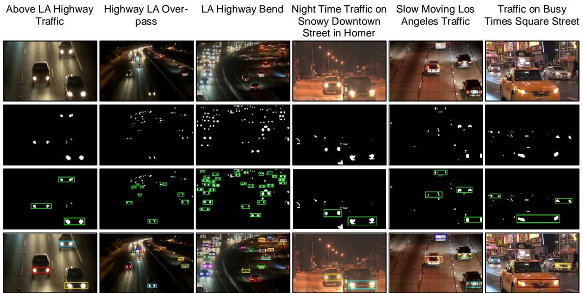
Fig. 5. Moving vehicles tracking in highway and urban road traffic scenes of the dataset
