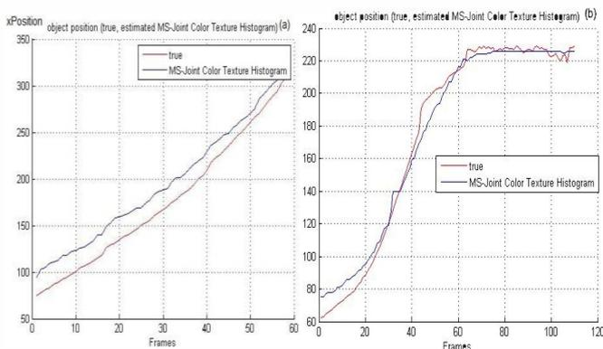
Fig. 6: Tracking trajectory for the video sequence 1 (a) and video sequence 2 (b) using MS-Joint-color texture histogram tracker.
