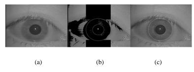
Figure 3. Iris localization and segmentation process (a) the original iris image (b) the region of interest (c) the segmented iris image
