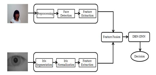
Figure 1. The block diagram of the proposed biometric system
